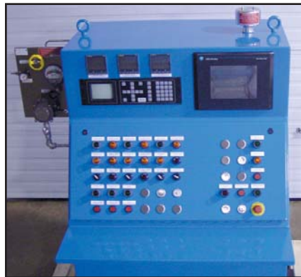
Operator's Control Console w/ touchscreen HMI
